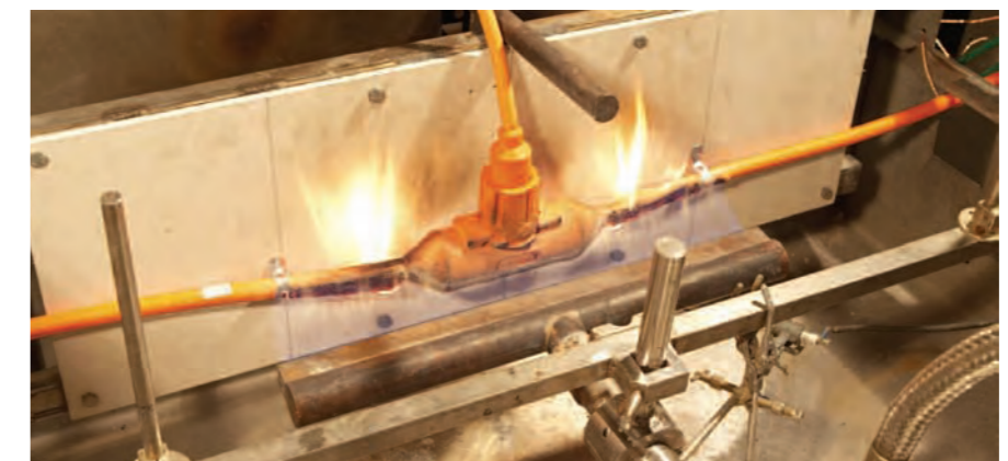
BS6387 Category Z - Resistance to fire with mechanical shock; 950°C for 15 minutes with 30 second hammer blows
